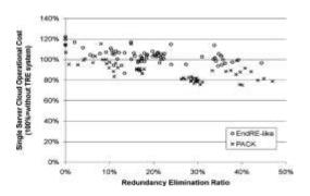
Fig 3: PACK versus End RE-like cloud server operational cost as a function of redundancy ratio.
